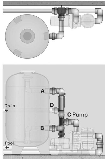
Besgo valves (DN65 / DN80 / DN100) should be attached to the wall on site using pipe clamps.
